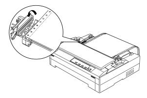
1. If you are using the front push tractor, remove the front cover.
